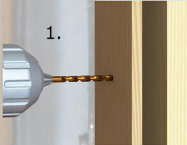
1. Predrill window frame/ door jamb (only) with 5/16" drill bit.
