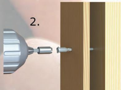
2. Engage crown bit into TopStar™ screw head and drive flush to surface of frame or jamb.
