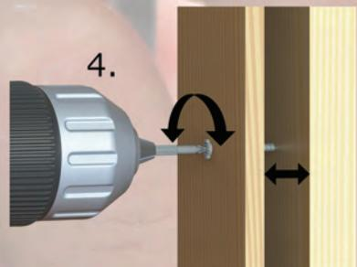
4. Engage bit into center hole of TopStar™ screw head and adjust to your requirements.
