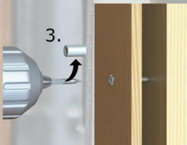
3. For adjustments remove crown from bit.
